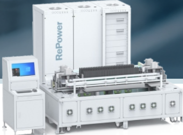
Solid-State Battery Capacity Grading System
